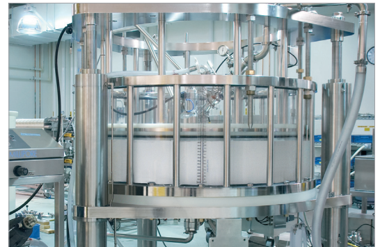
Large scale column (1.6 m) packed with ProSep® media
