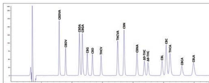
Figure 2. Separation of Cannabinoids in the Peak Identification Mix Using a Gradient on a 2.7 µm Ascentis® Express C18 Column
