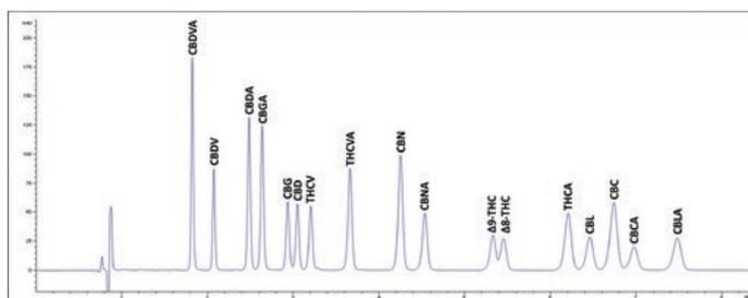
**Figure 3.** Separation of Cannabinoids in the Peak Identification Mix Using an Isocratic Method on a 2.7  $\mu\text{m}$  Ascentis<sup>®</sup> Express C8 Column.
