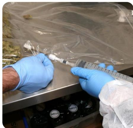
**Figure 4.** Indoor profile measurement of cannabis terpenes using headspace on dried plant materials placed in a bag (e.g. Tedlar® gas sampling bag) using a stainless Carbotrap® T420 TD tubes and large syringe to pull the sample through the tube. (when using a gas sampling bag, the tube in a TDS3™ container - equipped with sampling caps - can tightly be
