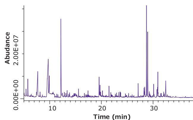
in sensitivity (**Figures 3 and 4**). The initial extraction time used was 20 min, and a shorter extraction time of 10 minutes was evaluated. However a loss in sensitivity was noted, thus extraction time was maintained at 20 minutes. The DVB/CAR/PDMS fiber was then evaluated (**Figure 5**). As expected, this fiber extracted more of the lighter compounds, which by MS spectral match, were identified as short chain alcohols and acids.
