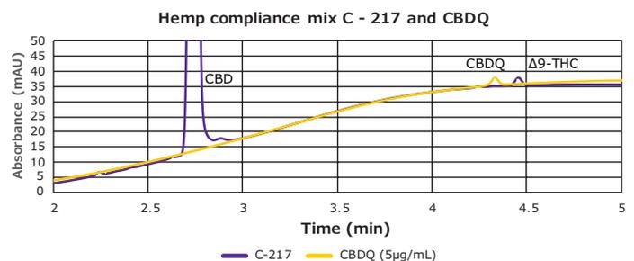
**Figure 4:** Overlay of HPLC-UV chromatograms of C-217 hemp compliance mix and a solution containing CBDQ.
