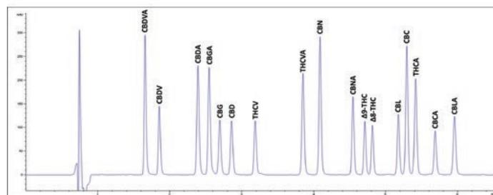
Figure 1. Separation of Cannabinoids in the Peak Identification Mix Using a Gradient on a 2 µm Ascentis® Express C18 Column
