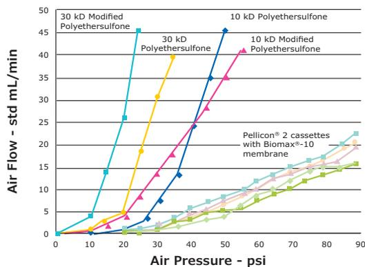
**Figure 6.** Integrity test comparison-air flow through wetted cassettes
