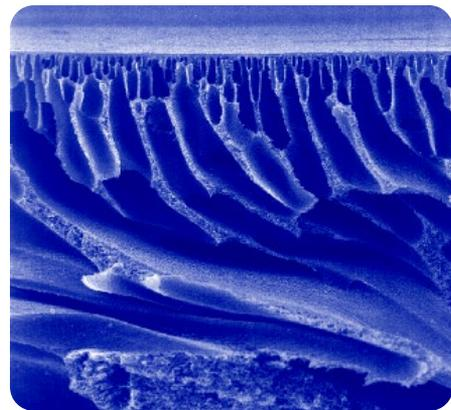
**Figure 2.** Conventional 10 kD polyethersulfone membrane with sub-surface voids
