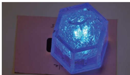
Figure 12. Check of Electrical Conductivity of Polypyrrole Thin Film Using Crystal Candle
