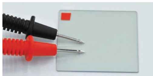
Figure 11-1. Check of Conducting Plane on ITO Glass
