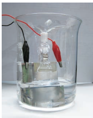
Figure 10. Synthesis of Polypyrrole by Electrochemical Polymerization
