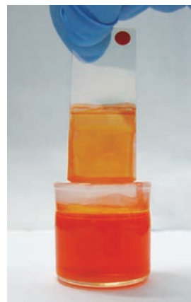
Figure 14. Dip Coating with MEH-PPV (Luminescent Layer)
