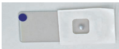
Figure 15-2. Preparation of Gallium-Indium Eutectic Mixture (Electron Injection Layer)
