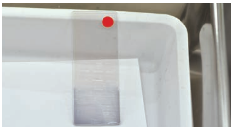
Figure 13-5. Drying of PEDOT Thin Film (Hole Injection Layer)
