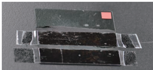
Figure 11-4. Fixation of Polypyrrole Thin Film
