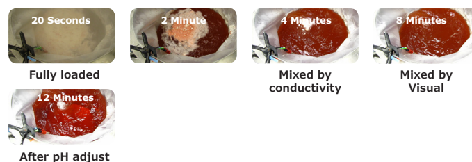
Figure 5. Ex-Cell® Advanced™ Medium mixes quite efficiently in the Mobius® Power MIX 100. Conductivity reaches a stable value at 4 minutes, with only a small amount of powder still undissolved. The last of the powder is incorporated at 8 minutes for complete visual mixing. Particle count also levels out between 5 to 10 minutes. After pH adjustment, conductivity increases slightly and particle count goes to minimum. Finally, with Q.S. to 100 L, conductivity is decreased, while particle count and pH remain constant.
