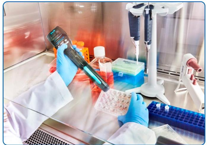
**Figure 9.** Scepter™ 3.0 handheld cell counter.
