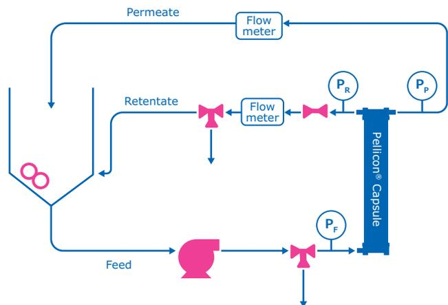
**Figure 1.** Schematic of TFF system setup.
