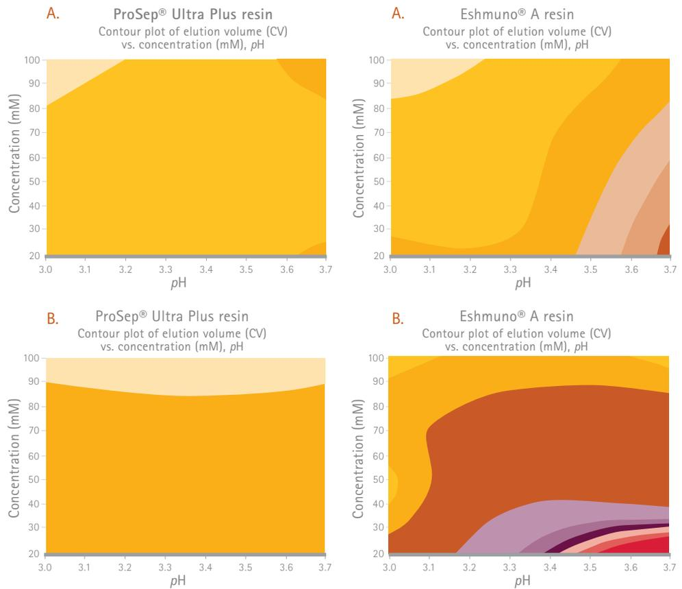
**Figure 1.** Elution pool volume using citric acid (A) and acetic acid (B) as the elution buffers on ProSep® Ultra Plus (left) and Eshmuno® A (right) affinity resins.
