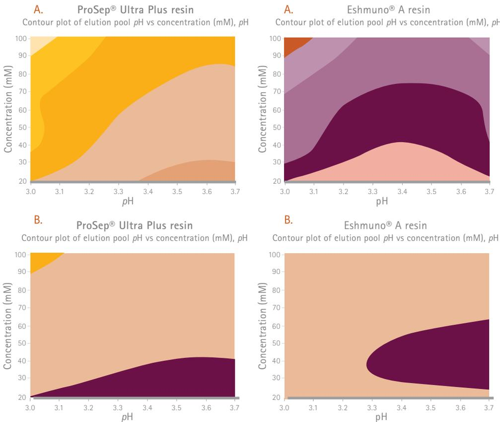
**Figure 2.** Elution pool pH using citric acid (A) and acetic acid (B) as the elution buffers on ProSep® Ultra Plus (left) and Eshmuno® A (right) affinity resins.
