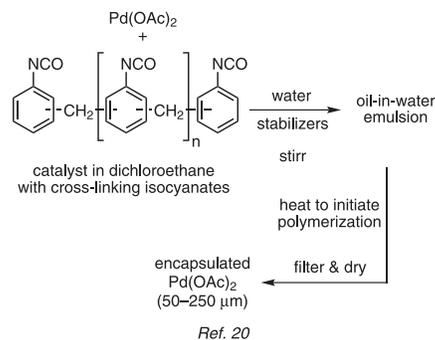
**Figure 1.** Interfacial Microencapsulation of Palladium in a Polymer Matrix.
