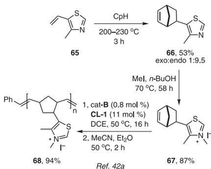
Scheme 11. Preparation of a High-Load, ROMPgel-Supported Thiazolium Iodide.
