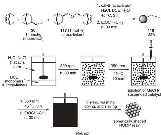
**Scheme 21.** Preparation of Spherical, Unsaturated ROMP (U-ROMP) Resins by Suspension-ROMP.
