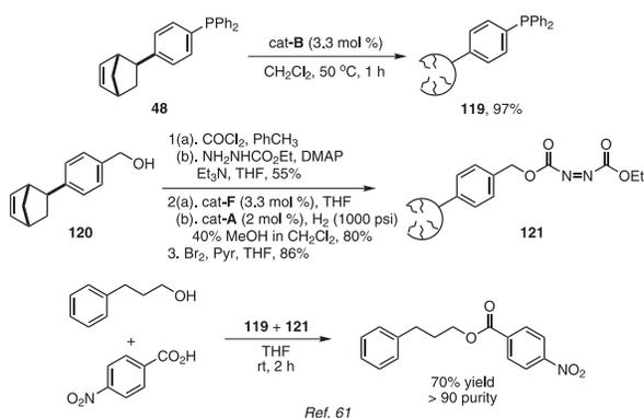
**Scheme 22.** Application of the Polymer-on-Polymer Approach in the Mitsunobu Reaction.
