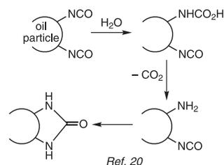
**Scheme 1.** The Polyurea-Matrix-Forming Reaction That Occurs at the Oil–Water Interface.
