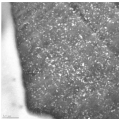
**Figure 2c.** Transmission Electron Microscope (TEM) Image of Ultramicrotone Cross Sections of Pd(OAc)<sub>2</sub>-Containing Microcapsules. (Photo courtesy of Avecia Ltd, and is reproduced with permission.)
