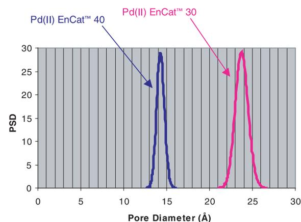
**Figure 3.** Pore Size Distribution (PSD) for Pd(II) EnCat™ 30 and Pd(II) EnCat™ 40 in the Tetrahydrofuran-Swollen State as Determined by Chromatographic Porosimetry. (Graph courtesy of Avecia Ltd, and is reproduced with permission.)
