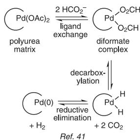
Scheme 2. Formation of Nanoparticulate Pd(0) via Ligand Exchange with the Formate Anion.
