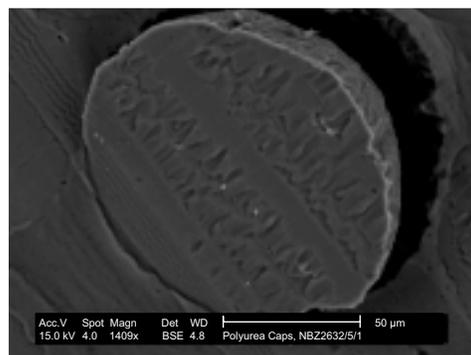
**Figure 2b.** SEM Image of the Interior of a Pd(OAc)<sub>2</sub>-Containing Microcapsule. (Photo courtesy of Avecia Ltd, and is reproduced with permission.)
