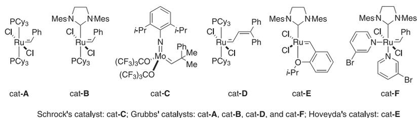
**Figure 1.** Examples of the Most Widely Used Olefin-Metathesis Catalysts.
