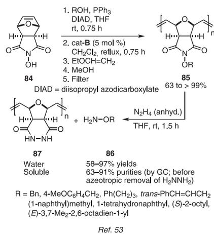
Scheme 14. Illustration of the Capture–ROMP–Release Approach to Product Purification.
