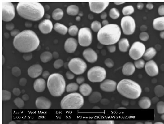
**Figure 2a.** Scanning Electron Microscope (SEM) Image of Microcapsules Containing Pd(OAc)<sub>2</sub>. (Photo courtesy of Avecia Ltd, and is reproduced with permission.)
