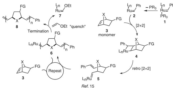
**Scheme 1.** Mechanism of ROMP.
