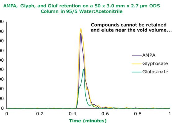
**Figure 3.** Three Polar Pesticides on an ODS Stationary Phase. No separation occurs and the compounds elute at or near the void volume of the column.
