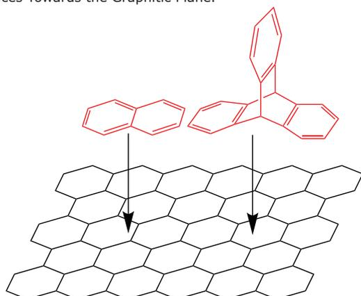
**Figure 2.** Representation of Analyte (red) Alignment with the Graphitic Surface (black). Analytes that can align their surface area flat against the graphitic plane have a stronger Interaction and tend to retain for longer as a result. More surface area contact attributes itself to longer retention than less surface area contact. An example illustrated here is naphthalene (left, stronger interaction) vs triptycene (right, relatively weaker interaction although one additional aromatic ring).
