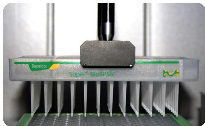
**Figure 2.** Supel™ BioSPME 96-Pin Device Maneuvered by Automated Liquid Handling System Gripper.
