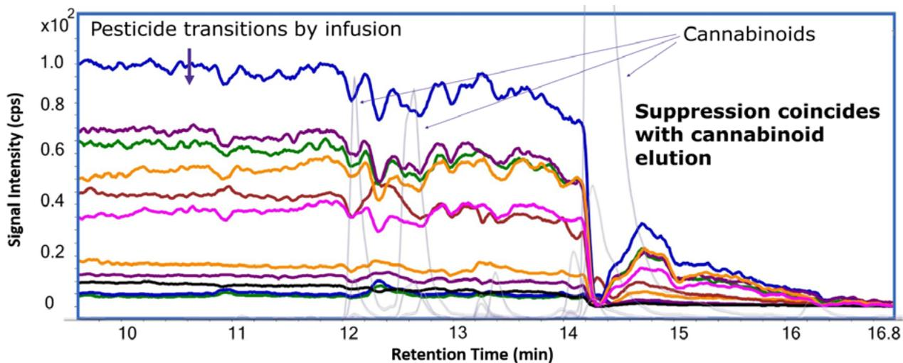
**Figure 4.** A portion of the Chromatographic Run in a Tee-Infusion Experiment - The colored traces indicate the signal intensity of several pesticides being infused over the course of a run. The cannabinoid peaks (grey) were collected as a separate chromatographic run and have been overlaid with the infusion data for illustration. The suppression occurring after 15 minutes is due to unidentified matrix components eluting from the column.
