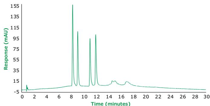
**Figure 9.** Separation of 25-Hydroxyvitamin D2 and D3 and Their Epimers on Supel™ Carbon LC. Elution order:
