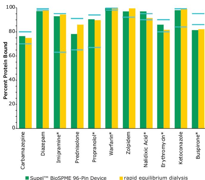
**Figure 4.** Comparison of Protein Binding Values Between Supel™ BioSPME 96-Pin Device and Rapid Equilibrium Dialysis Methods. The blue lines indicate the published protein binding literature value intervals. Compounds with asterisks are charged at physiological pH.
