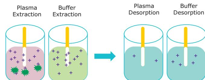
**Figure 3.** Representation of the extraction step (left) removing free analytes from plasma (pink) and buffer (green) and the analytes releasing into the desorption solution (blue).
