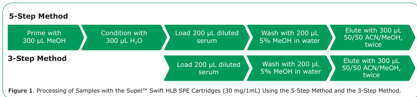
Figure 1. Processing of Samples with the Supel™ Swift HLB SPE Cartridges (30 mg/1mL) Using the 5-Step Method and the 3-Step Method.
