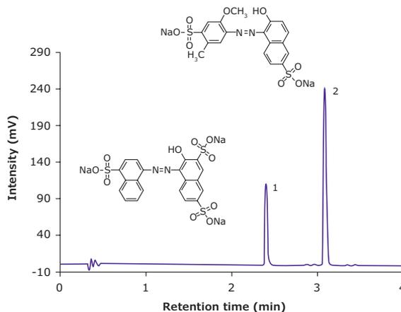
Analysis of colorants in rum. Two food colorants in rum, E 123 (Amaranth) and E 129 (Allura Red AC), were analyzed to illustrate the long-term performance and method robustness of Chromolith® columns. More than 8,000 samples (total volume of injected sample: 16 mL + 30 L mobile phase) were analyzed on a 50 x 2.0 mm Chromolith® RP-18 endcapped column.
