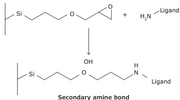
Reaction between epoxide functions on monolithic surface with amines forming a secondary amine bond
