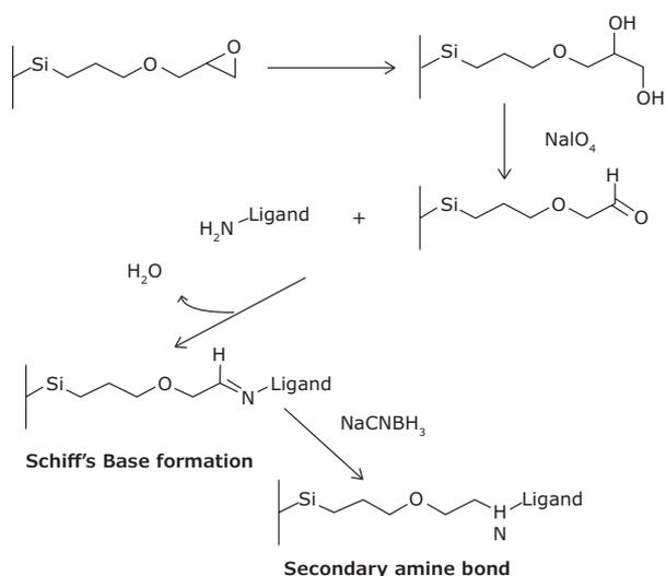
Scheme of immobilization via Schiff base mechanism.
