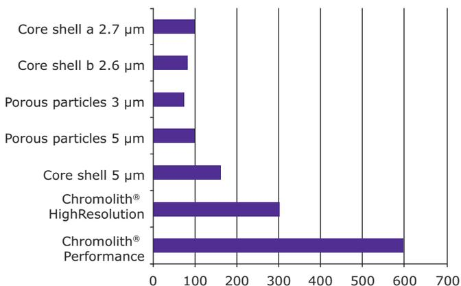
All columns are C<sub>18</sub> modified, 100-4.6 mm. Sample: anthracene, eluted isocratically using acetonitrile/water (60/40) at 2 mL/min flow rate. Injection volume: 5 µL, detection at 254 nm UV. All analyses performed at room temperature.
