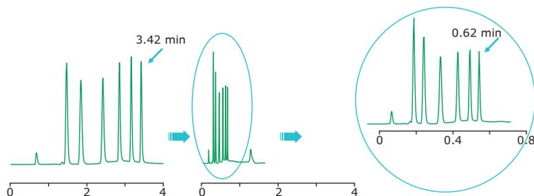
Column: Chromolith® FastGradient RP-18e 50-2 mm; Mobile phase: [A] Water, [B] Acetonitrile; Gradient;
