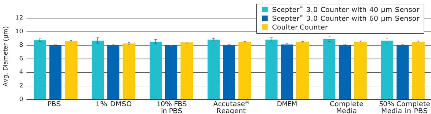
Polystyrene beads of known diameter (8 µm) suspended in various cell culture buffers and reagents were measured using the Scepter™ 3.0 Cell Counter with both 40 µm and 60 µm sensors. Results are compared to the same counts obtained with a Coulter Counter Z2™ Instrument equipped with 100 µm aperture. Data are from three measurements per sample.
