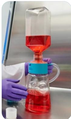
Stericup® E and Steritop® E filters thread directly onto any commercial media bottle or glass bottle:
