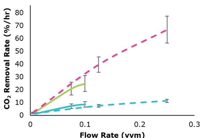
— 3 L Open Pipe    — 200 L Open Pipe    — 200 L Drilled Hole Sparger    - - 3 L Microsparger
