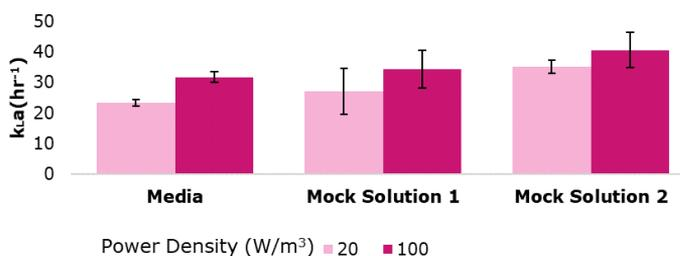
**Figure 8.** For the microsparger, a 1 X PBS solution (Mock Solution 1) is closest to the cell culture media  $k_La$  performance, and therefore characterization data from this solution would be more appropriate to use to estimate VCD. Data is the average  $\pm$  SD of n=2 Mobius® 3 L Single-Use Bioreactors.
