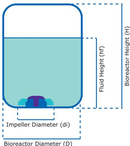
**Figure 1.** Key for bioreactor geometry in **Table 1.**
