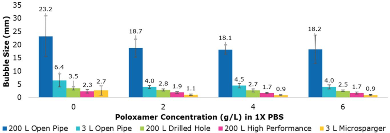
Figure 9. Bubble size characterization of newly designed Mobius® iFlex Bioreactor 50 L – 200 L spargers (open pipe, drilled-hole, high performance) compared to Mobius® 3 L Bioreactor spargers among several mock media formulations. Error bars are standard deviations.
