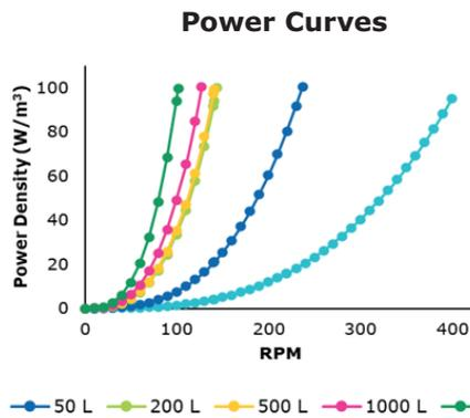
**Figure 3.** Power curves from 3 L to 200 L. Each reach > 90 W/m<sup>3</sup> within operating range of rpm at full volume.
