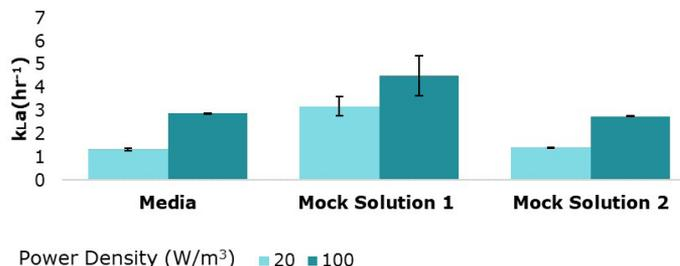
**Figure 7.** For the open pipe sparger, a 1 X PBS 4 g/L EMPROVE® Poloxamer 188 50 ppm EX-CELL® Antifoam C solution (Mock Solution 2) performs more similarly to media  $k_La$ , and therefore characterization data from this solution would be more appropriate to use to estimate VCD. Data is the average  $\pm$  SD of n=2 Mobius® 3 L Single-Use Bioreactors.
