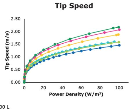
**Figure 4.** Tip speed per power density 3 L to 2000 L. All impellers achieve <2.2 m/s at >90 W/m<sup>3</sup> at full volume.
