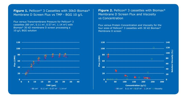
Scalability was assessed using two methods. The model protein stream was BGG in phosphate buffered saline, pH 7.1. Three Pellicon® 3 cassettes with 30kD Biomax membrane and D screen, from each size, were randomly selected to provide a sample representation of the available cassettes (Table 1).
