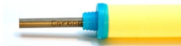
After sampling, the cartridge adsorbent is placed in a TD empty tube and analyzed by thermal desorption (TD)/GC-MS. Read more about this sampling on our website [SigmaAldrich.com/radiello](http://SigmaAldrich.com/radiello).
