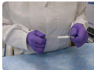
After sampling, insert the DSD device back into its original storage container.
