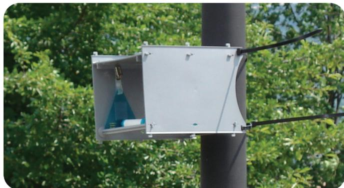
The protective outdoor shelter is easily transported and assembled directly at the sampling site.
