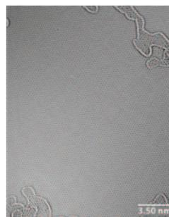
**Figure 6.** HRTEM image of a CVD monolayer graphene film ([Aldrich Product Nos. 773697, 773700 and 773719](#)) produced in Graphenea.
