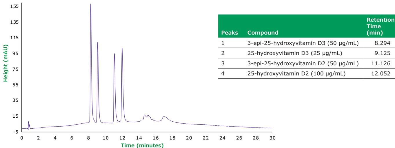
**Figure 2:** Chromatographic separation of Vitamin D2 and D3 metabolites on Supel™ Carbon LC. Conditions: Column: Supel™ Carbon LC, 10 cm x 2.1 mm I.D., 2.7 µm; Mobile Phase: [A] 2-Propanol; [B] Tetrahydrofuran; Gradient: 0% B to 70% B in 15 min; hold at 70% B for 5 min; Flow Rate: 0.3 mL/min; Column Temp.: 25 °C; Detector: UV, 275 nm; Injection: 2.0 µL; Sample: Vitamin D2 and D3 metabolites mix, varied concentration, ethanol
