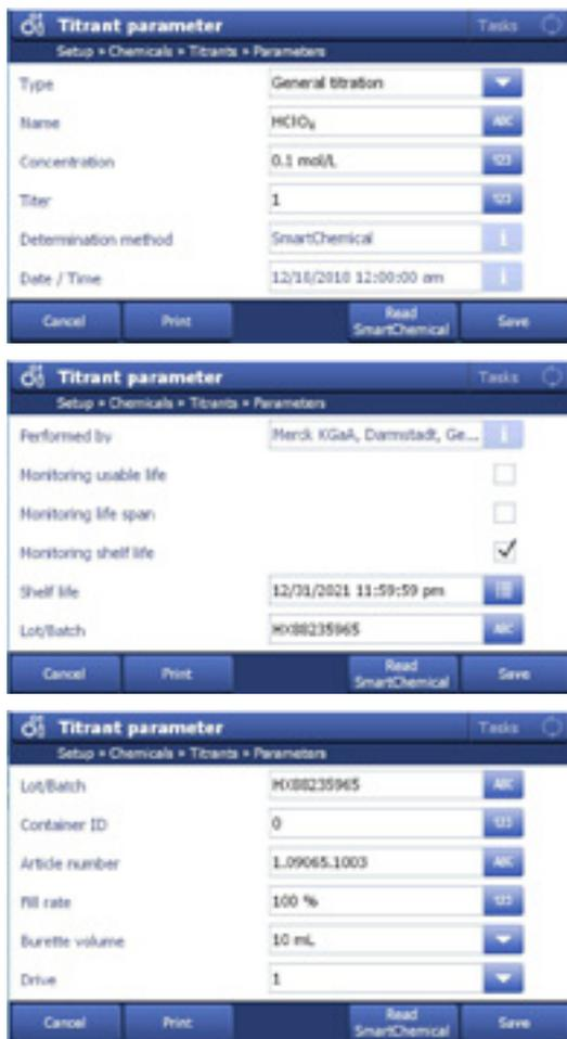
Figure 3. Information on SmartStandards as displayed in the titrator software
