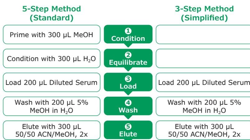
**Figure 1.** General processing of samples (serum 1:1 diluted) with *Supel<sup>™</sup> Swift HLB cartridges* (30 mg/1 mL) using a 5-step method and a 3-step method
