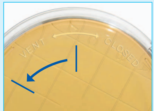
Turn lid counter clockwise and click in VENT -position
