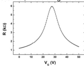
Typical transfer curve measured at  $V_{SD}=20mV$  (right), measured at room temperature in vacuum.
