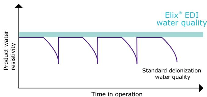
With Elix® EDI technology, deionization quality and cost remain constant, and are independent of feed water quality, RO membrane efficiency, and pure water use.
