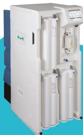
Milli-Q® CLX 7000 systems can deliver up to 3000 L/day of CLRW to analyzers by automated feed.
