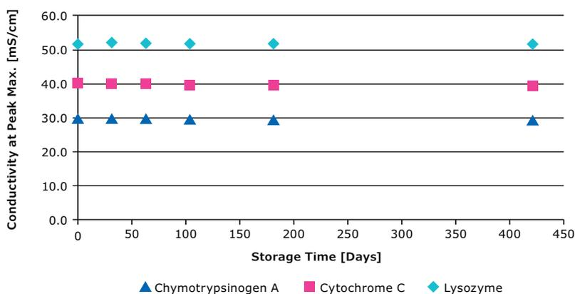
**Figure 9:** Elution conductivities at peak maxima for a standard separation on a packed column (100 mm x 16 mm i.d., 12% compression) stored in 1.0 M sodium hydroxide for certain times after re-equilibration.
