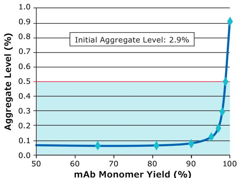
**Figure 6.** Eshmuno® CPX -HCP, leached protein A, and aggregate clearance.
