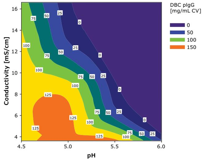
**Figure 2.** Flow packed in 0.15 M sodium chloride, 20 cm bed height, 15% compression, running buffer: 0.15 M sodium chloride. Static binding capacity of mAb07 across conductivity ranges of 5–12 mS/cm and a pH range of 4.00–5.25. The color scale represents the binding capacities, at various pH and conductivity ranges.
