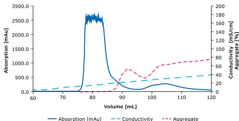
**Figure 5.** mAb aggregate % removal during linear salt gradient elution.
