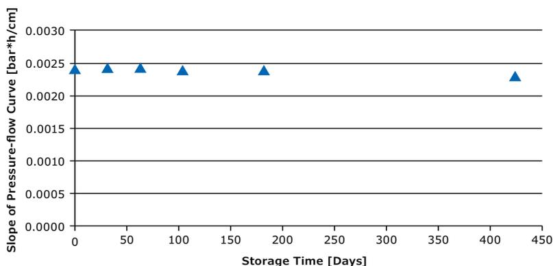
**Figure 10:** Pressure versus flow curves were recorded in 100 x 16 mm i.d. columns packed to 12% compression (150–1500 cm/h) after treatment with 1.0 M sodium hydroxide for certain times. The slope of the net pressure drop versus flow curve after treatment with 1.0 M sodium hydroxide for certain times was determined by linear regression. The coefficient of determination ( $R^2$ ) was always greater than 0.995 indicating a strong correlation between the variables.
