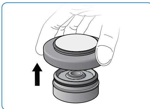
Figure 18: Filtration unit base removal
