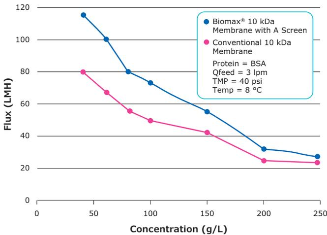
Figure 1. High flux of Biomax® membrane versus conventional polyethersulfone UF membrane.
