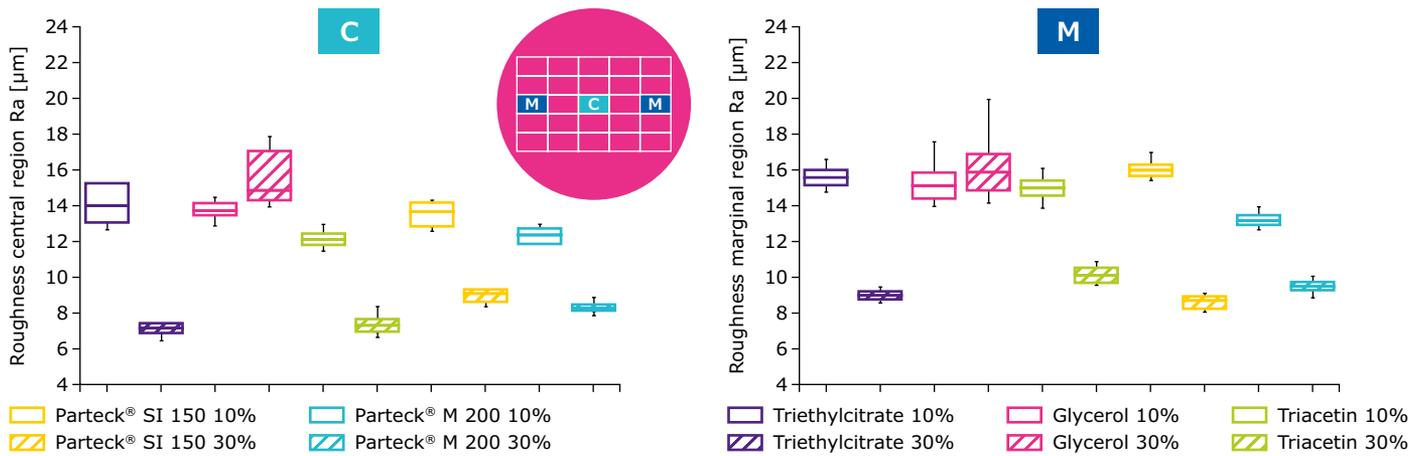
**Figure 8.** Influence of different plasticizers on the roughness of the tablet surface measured in the center (C) and margin region (M) of the tablet.
