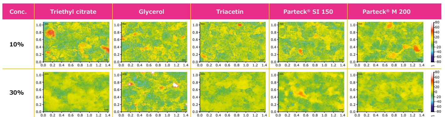
**Figure 9.** Effect of different types and concentrations of plasticizers on tablet surface roughness.
