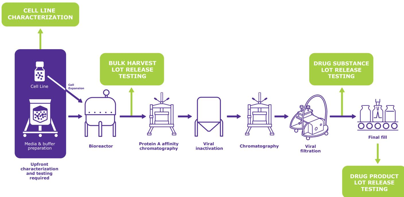
**Figure 1.** Current manufacturing processes utilize batch operations that require biosafety testing across the whole process
